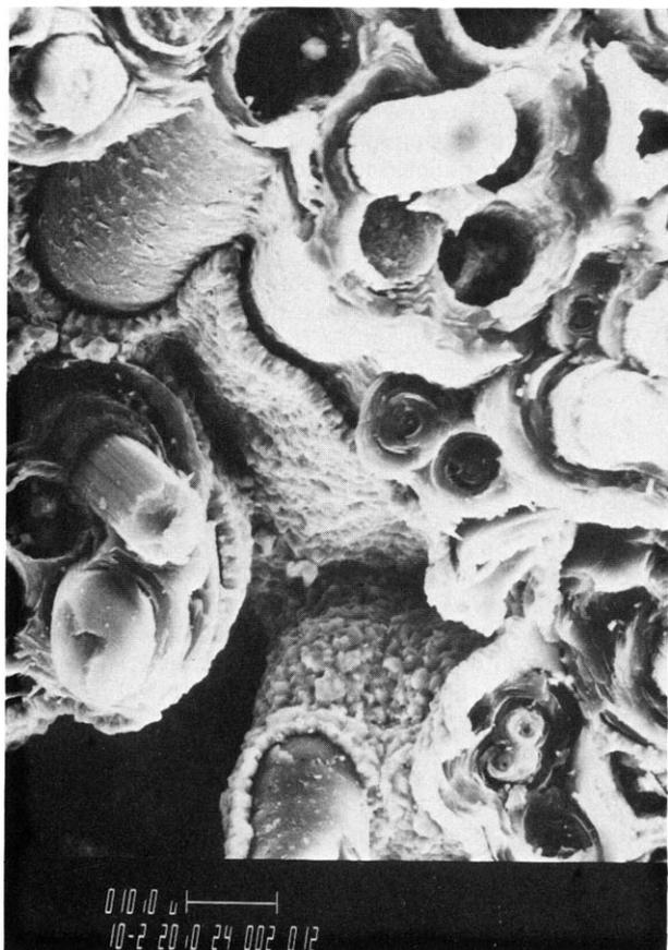
Fig. 17. SEM fractography of a composite type 4.
